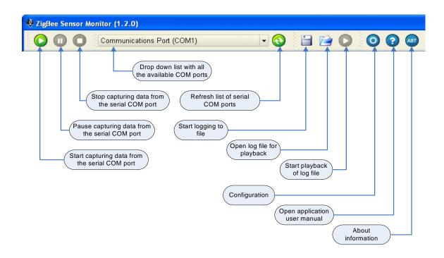
The list of available COM ports will automatically be updated when the eZ430-RF2480 dongle is connected or disconnected. It is also possible to force refresh of the list by clicking on the green "refresh" button ③.
